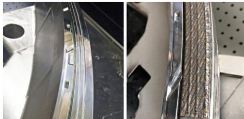
Whether it is cutting or forming, the Hybrid 3D printing method is capable of repair metal products that have worn down, thanks to its ability to be molded directly onto metal, no matter what process it has already undergone previously. The connecting rod trim punch repair case, where service life increased more than twofold from 20,000 ~ 60,000 shots to 150,000 after worn-down parts were repaired using InssTek's DMT® printing, proves the effectiveness of Hybrid 3D printing.
