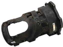
cost of replacing 12 parts by saving more than KRW 100 million (USD 100, 000), and also shortened the maintenance period by 75%. The repair of the Vulcan cannon of the Army Maintenance Depot is another example. The Vulcan cannons are disposed when the gun housing is worn out. Constant wear of the gun housing means Vulcan cannons consume considerable amounts of time and cost. With 3D printing technology, the worn out parts can be repaired using the same metal powder, saving time and money.
